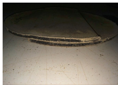
Figure 2: Joint after test. No root penetration
