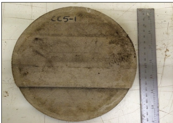
Figure 5. CC5-1 After the test (upper surface), no root penetration
