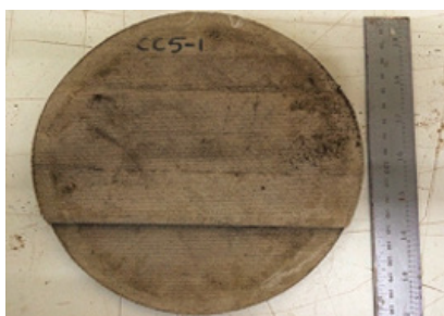
Figure 1: Upper surface after test. No root penetration
