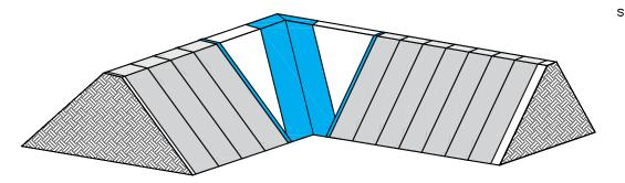
Stage 4 — Deploy valley CC/CC Hydro cover layer, jointing to top surface of valley CC Hydro layers by thermal bonding along all edges using minimum 60mm perforated slot nozzle.
