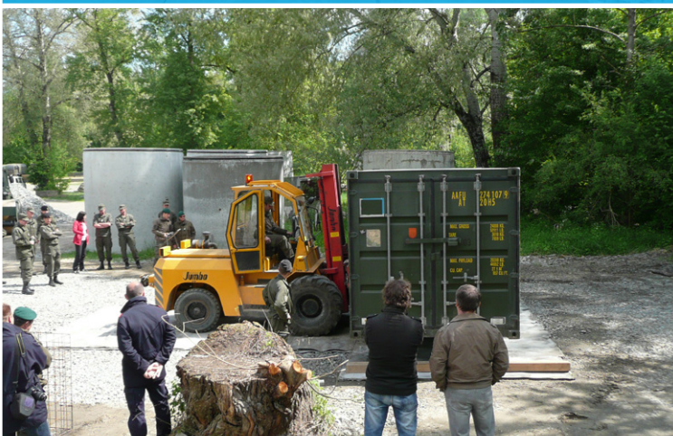
13T load driven onto hardened CC trackway
