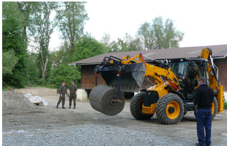
CC13™ Bulk roll on spreader beam
