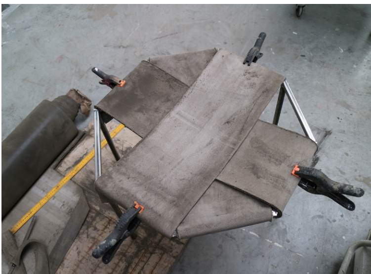
Edges of the small table clamped to keep shape following hydration
