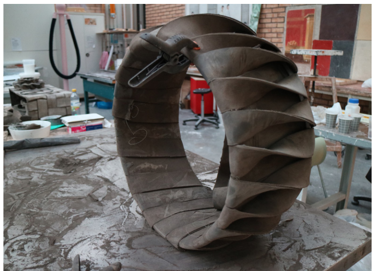
Planter pot hydrated and clamped to allow the CC to set
