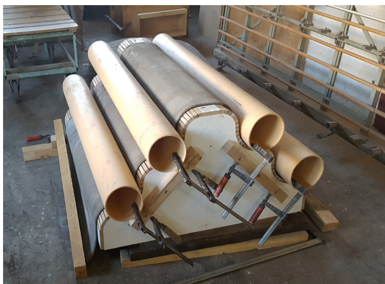
The CC was shaped, hydrated and left to set
