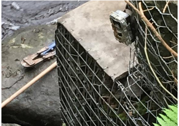
CC attached to gabion baskets using hog rings
