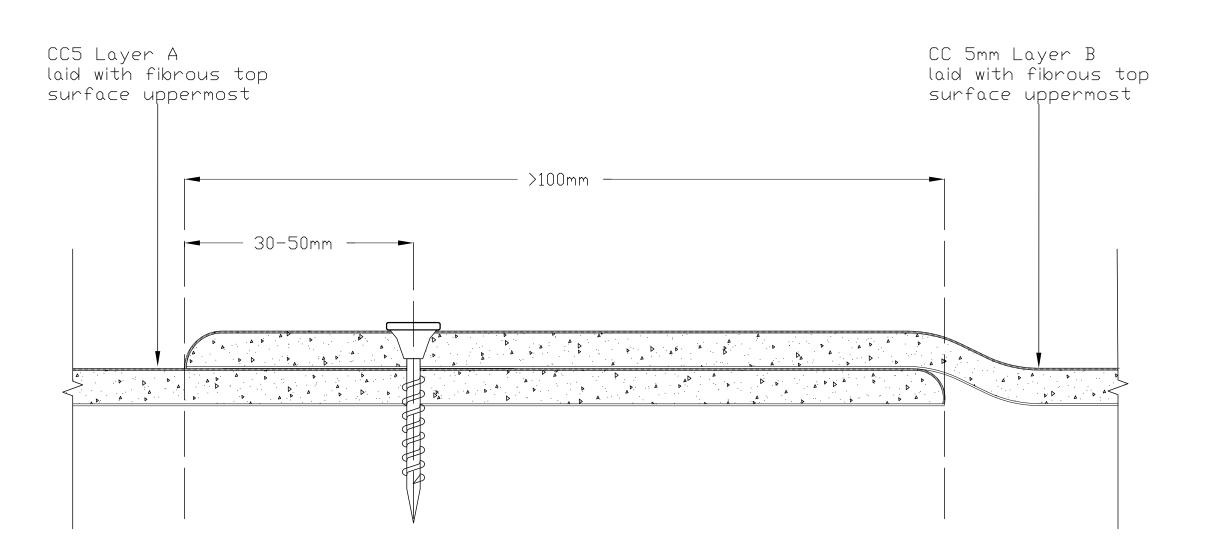
NDTE: CC jointing detail above is not impermeable and is designed to be used only for non containment applications to provide erosion control and weed supression.
