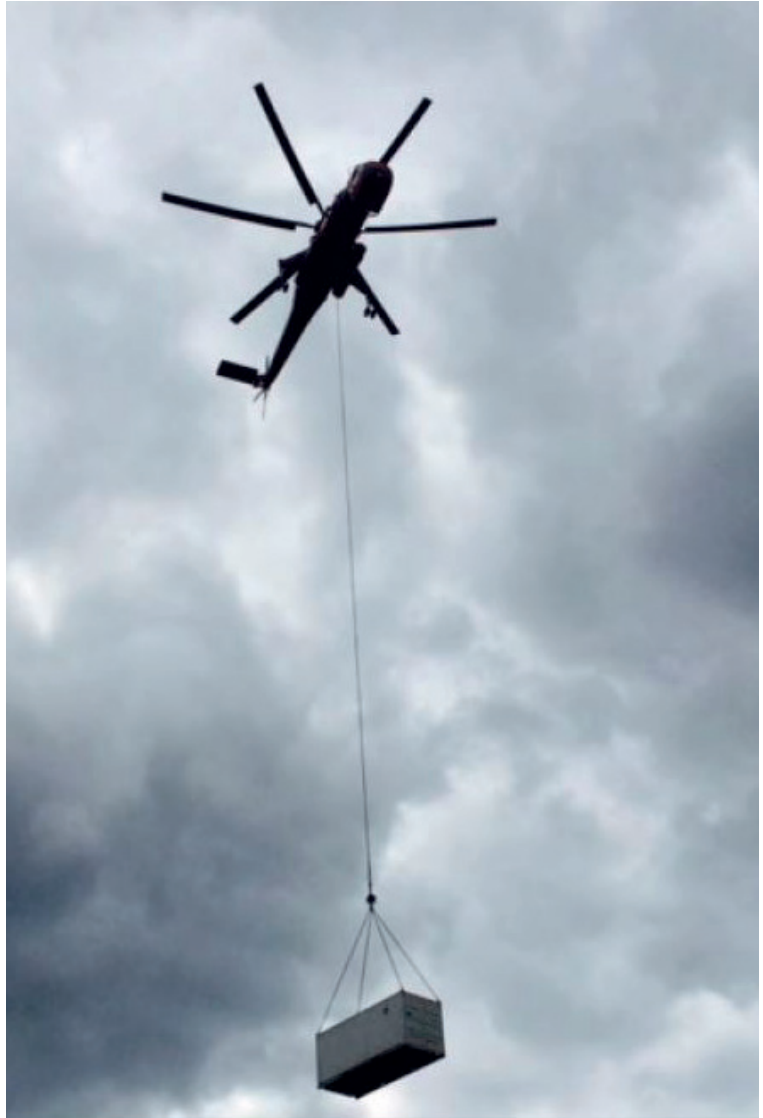
CC bulk rolls were airlifted to site
