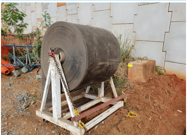
Bulk roll on standing frame-mounted spreader beam for deployment
