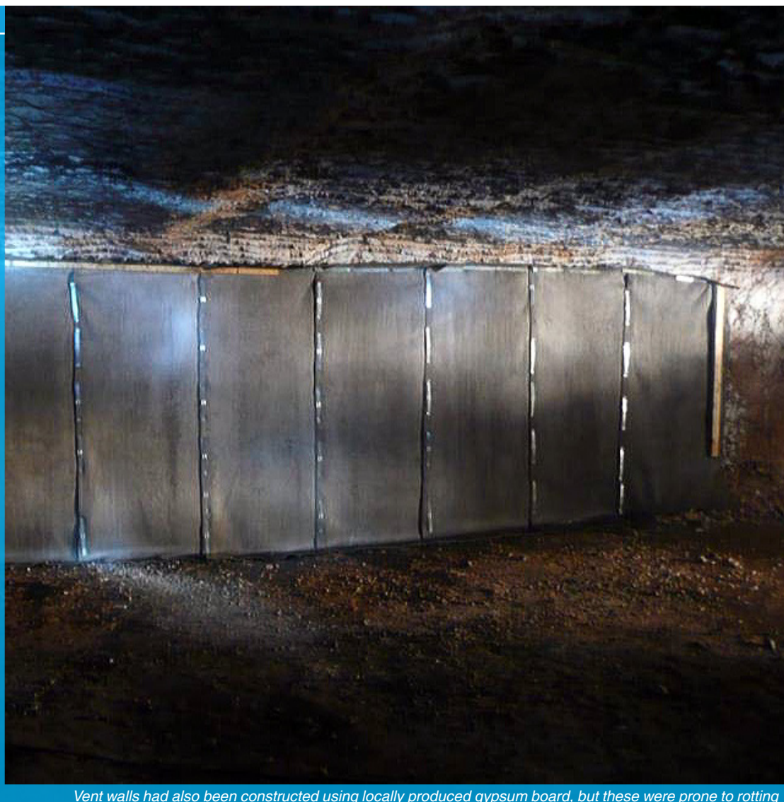
Vent walls had also been constructed using locally produced gypsum board, but these were prone to rotting
