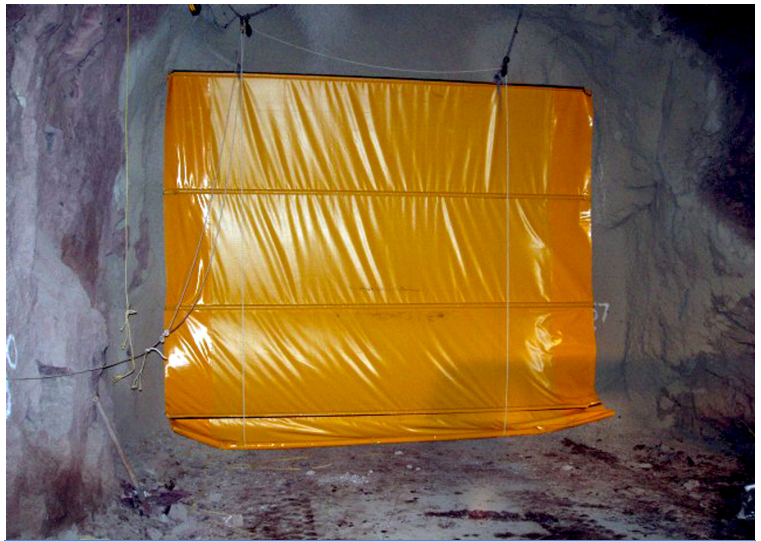
Brattice cloth had also been used but only as a temporary measure
