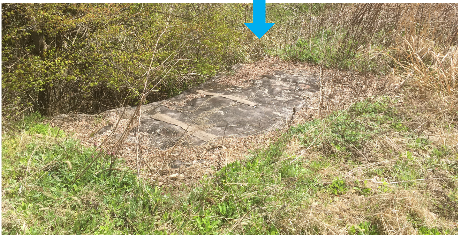
Day 816 - CC is beginning to moss over with age and still shows no signs of weed protrusion
