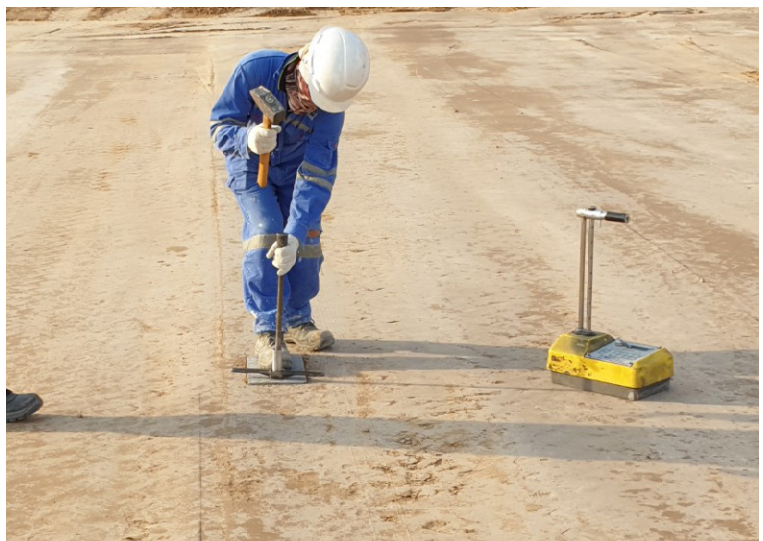
Compaction testing of marl base
