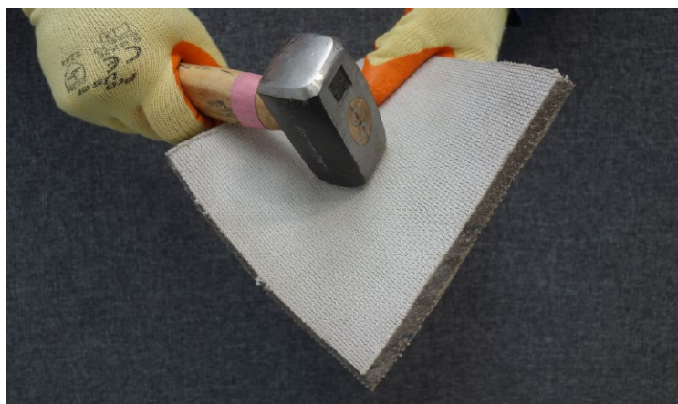
Figure 1. The change of GCCM properties from flexible to rigid on curing means that when assessing GCCM properties, appropriate test methods should be used to determine the cured, in-service GCCM cementitious layer performance.
